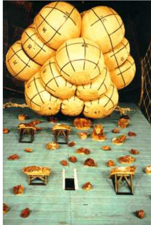
Figure 10: Pathfinder airbags being dropped onto a rocky and inclined plane to simulate landing on Mars. http://mars3.jpl.nasa.gov/MPF/mpf/mpfairbags.html
