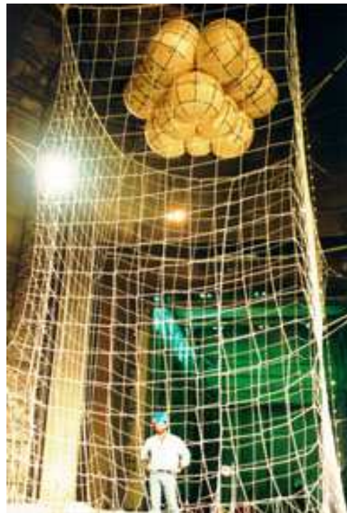
Figure 11: Airbags being prepared for testing, with person for scale. http://mars3.jpl.nasa.gov/MPF/mpf/mpfairbags.html
