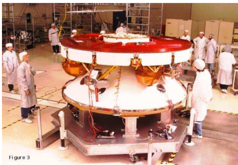
Figure 3: Pathfinder's cruise stage (top) and aeroshell (bottom) prior to launch. http://mars.jpl.nasa.gov/MPF/nasa/figstabs/figures/
